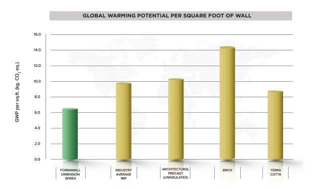
Examining the data above, Insulated Metal Panels (IMPs) on average contain less embodied carbon than precast concrete and brick, and Formawall Dimension Series in particular performs even better. Dimension Series contains less than half of the embodied carbon content of brick, and 36% less than architectural precast concrete.
